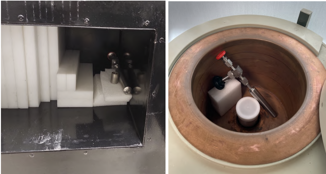
Figure B.1: Left : The nano-CaO powder container next to the Am-Be source inside a PE shielding. Right : After irradiation, the container is placed inside the HPGe detector to examine the associated ^{42}\text{K} production.
