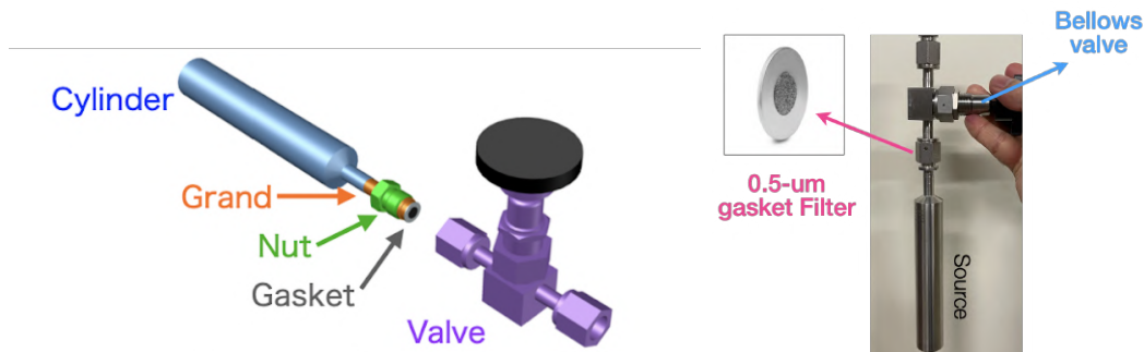
Figure B.2: The left diagram depicts Swagelok components housing CaO nano-powder, while the right image emphasizes the actual container, spotlighting the 0.5\ \mu\text{m} gasket filter and the bellows valve linking the container to the gas panel.
